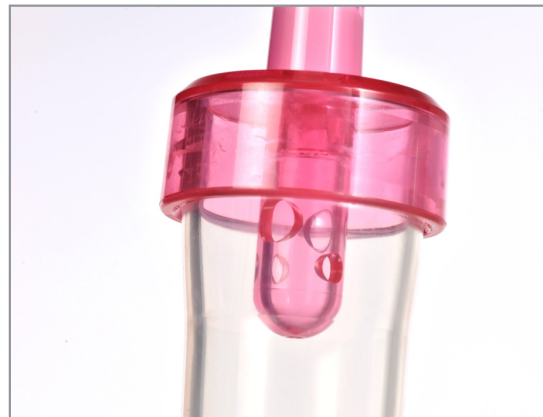
Bubbles and fogging are eliminated by perforations in the dispersing tube that flow evenly along the walls, while maintaining a good flow rate.
